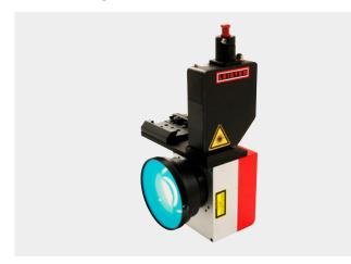
The Scanner Optic is characterized by the integrated option of motion and is mainly used for quasi-simultaneous welding. Two movable mirrors guide a spot-shaped laser beam along a programmed contour. The size of the working field can be adjusted by different focusing lenses. The Scanner Optic can be installed in various Leister laser welding systems.
