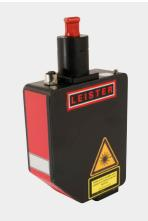
The Spot Optic focuses the laser beam to a spot and is mostly used for contour welding. The focal lengths of the focusing lenses used determine the spot diameter, which in turn determines the width of the weld seam. The laser beam can therefore be adapted to the individual requirements of plastics welding by replacing optical components.
