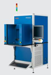
The laser welding system NOVOLAS<sup>™</sup> WS AT RTT is equipped with a rotary indexing table (RTT). The RTT increases throughput and efficiency by allowing the operator to safely load and unload components while components inside the system are being welded.
