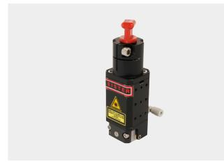
The Roller Optic does not require any additional clamping technology. In the Roller Optic, a line-shaped laser beam is guided through a glass roller, which is both the clamping tool and the last optical element. The double-sided roller can produce weld seam widths of around 3.0-6.7 mm. The roller's self-aligning bearing compensates for minor uneven spots in the axial direction.
