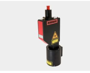
With the Radial Optic, rotationless radial welding is possible without additional clamping technology. Radial welding is suitable for rotationally symmetrical parts that are difficult to rotate themselves. The laser radiation is deflected onto the circumference of the parts by a conical mirror. This allows components with a diameter of up to Ø68 mm to be welded simultaneously. The advantages are short cycle times and high throughput.
