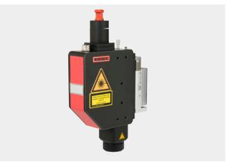
With the Globo Optic, welding in 2-D or 3-D is possible without complex clamping technology. The air-bearing glass sphere focuses the laser beam and serves as a mechanical pressure tool. As the ball rolls over the component, it presses permanently and locally on the joining plane. This means that the laser radiation only hits where contact pressure is present.
