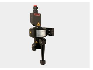
The Rotation Optic is used for the sequential welding of parts with rotational symmetry. It is operated solely with a fiber laser whose laser beam can be set to different spot diameters using an M-shape DOE. A synchronous electric motor with hollow shaft and incremental position measuring system is integrated into the optical system and moves an extension arm (rotor) around the part. At the end of the rotor, the laser beam is deflected towards the center using an adjustable mirror.
