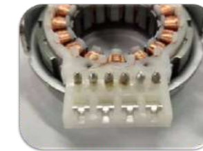
电机绕线柱 Winding pin Soldering
