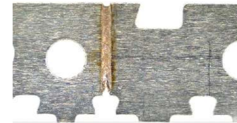
料带激光焊接 Material belt laser welding
