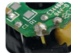
异型焊盘焊接 Deformed Pad Soldering
