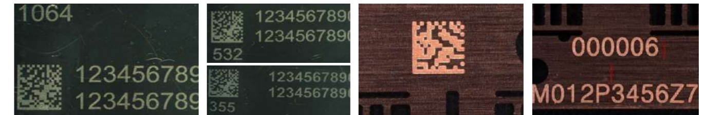
树脂打标效果(光纤、绿光、UV) After resin marking (fiber laser, green light, UV)
