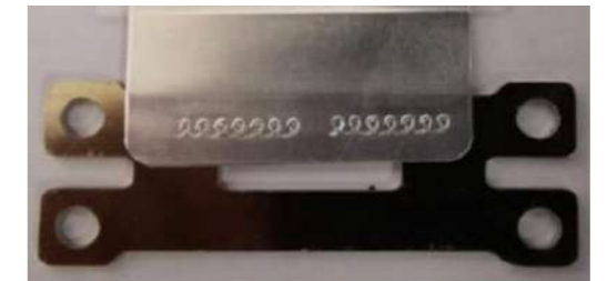
汇流排焊接 Bus bar welding
