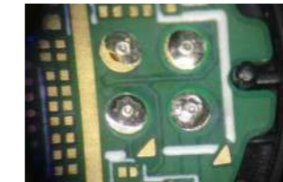
PCB过孔引脚焊接 PCB Punch Lead
